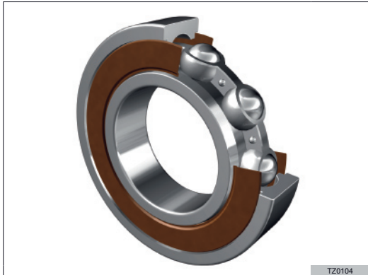
Fig.4 Single-row radial contact deep-groove ball bearing, sealed version with rubber seals on both sides
