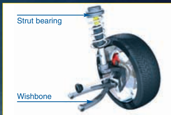
Wheel control pivots on the suspension strut where there is a bearing
