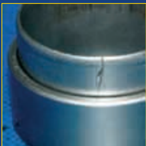
Outer damaged Forced fitting
